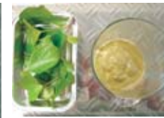
Leaves: Micro vial adapter plate / Micro vials / 3mm tungsten carbide bead per vial. Completely homogenized
