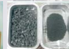
Rubber: 50ml steel jar / 20 mm steel Ball after cryogenic grinding
