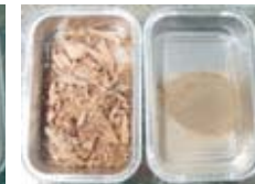
Wood / 50ml steel jar / 20 mm steel ball 200 Micron after 90 seconds
